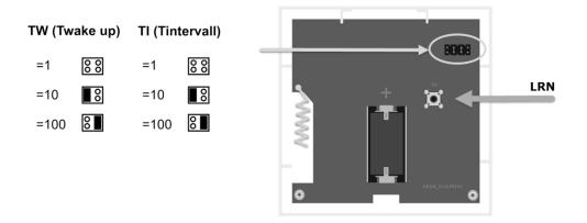
TW (Twake up): Measuring interval | TI (Tintervall): Transmission interval
