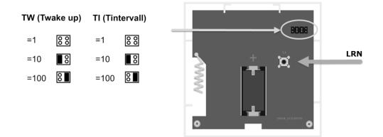
TW (Twake up): Measuring interval | TI (Tintervall): Transmission interval
