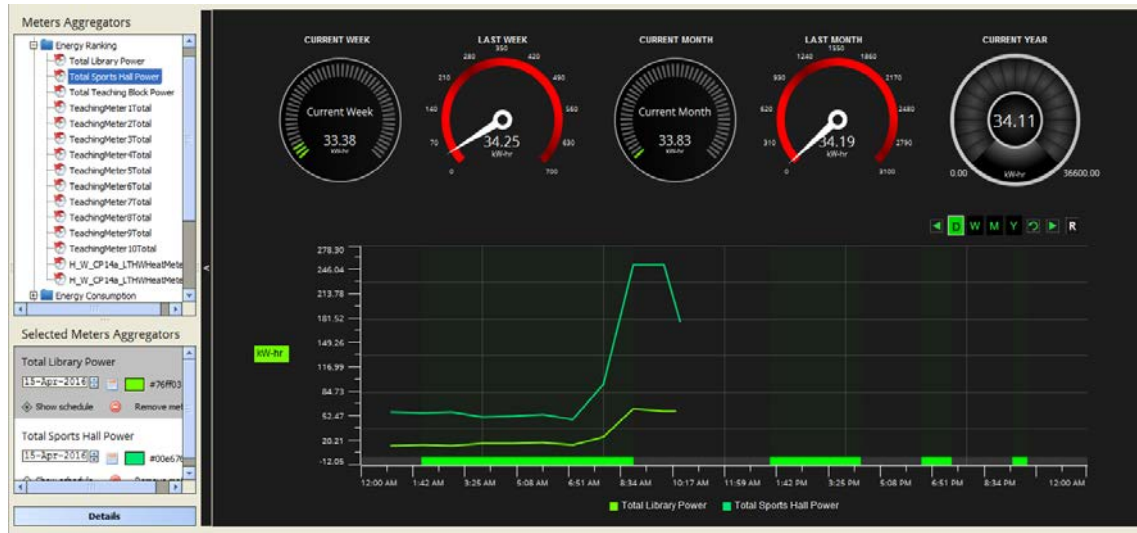
Figure 59 – Default view of the Meter Tree with two selected Meter Aggregators
