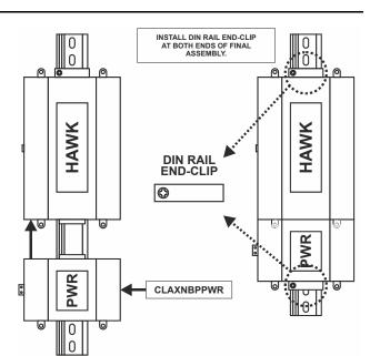
Fig. 2. Securing modules with end-clips
