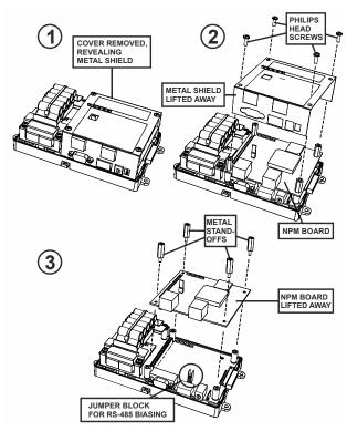
Fig. 11. Basic stages of controller disassembly.
