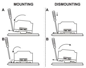
Fig. 1. Mounting/dismounting on DIN rail (recommended)
