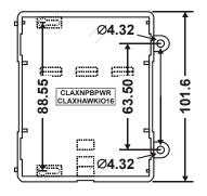
Fig. 5. Tab mounting of CLAXNPBPWR / CLAXHAWKIP16
