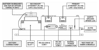
Fig. 9. HAWK (side view, cover removed).
