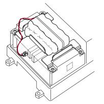
Fig. 13. Backup battery connector on HAWK 2xx/6xx bottom board.
