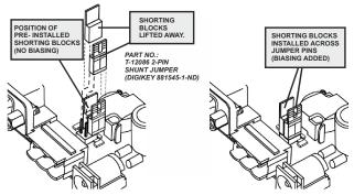
Fig. 12. Installing shorting blocks across both sides of the jumper block to add RS-485 biasing.
