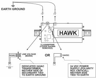
Fig. 8. CLAXNBPPWR module wiring connections.
