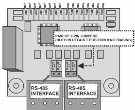
Fig. 10. Pair of 2-pin jumpers and corresponding RS-485 interfaces
