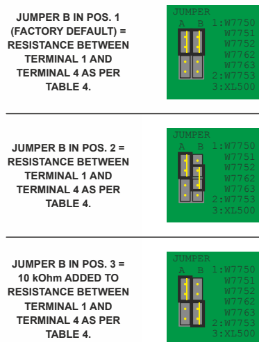
Fig. 6. Configuration of fan switch using jumper B
