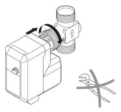
Fig. 3. Mounting the actuator
