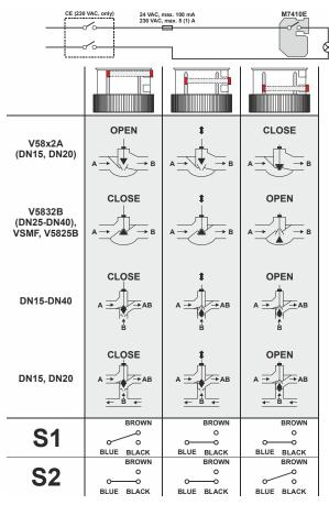
Fig. 10. Electric wiring of auxiliary switch
