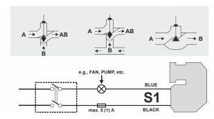
Fig. 12. Electric wiring of auxiliary switch
