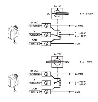
Fig. 5. Connection of input switch
