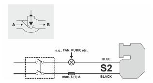
Fig. 11. Electric wiring of auxiliary switch
