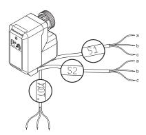
Fig. 8. Auxiliary switch cables
