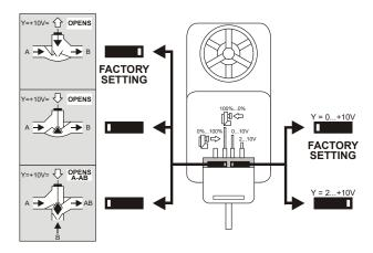
Fig. 4. Selecting valve type and output signal
