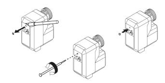
Fig. 9. Adjustment of auxiliary switch S2
