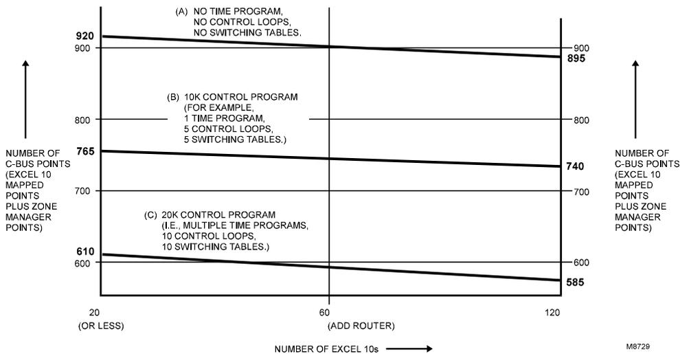
Fig. 21. Point capacity estimate for Zone Manager.
