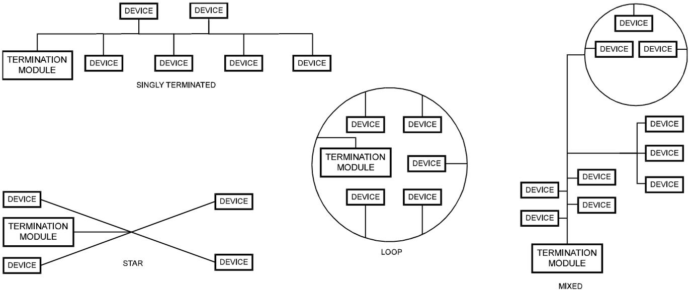
Fig. 12. Free topology E-Bus layout examples.
