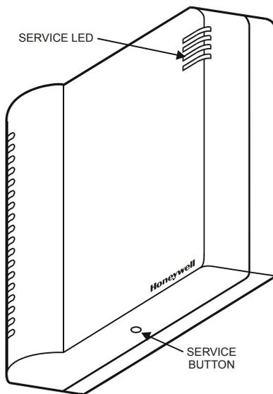
**Fig. 19. Hydronic Controller LED and service button.**
